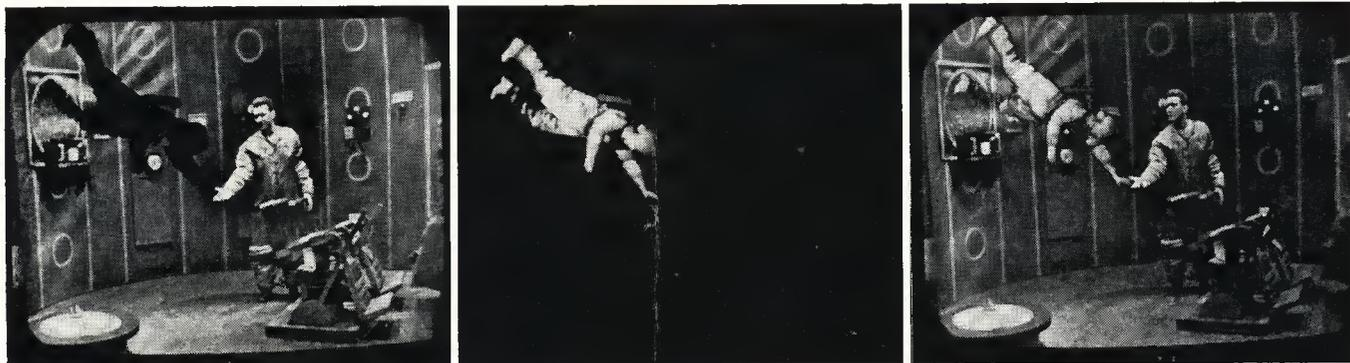
THE PHOTOGRAPHS above were taken off the camera monitors and clearly illustrate the action of the Gizmo. The picture on the first monitor shows the scene being picked up by that camera with the electronic cut-out of the image from camera two. The image on that camera's monitor is shown in the center. The figure is tilted with a prism. The combined picture is shown to the right. The imperfect picture is due to improper lighting and adjustment of the Gizmo. The finished product was much sharper.
